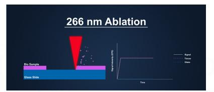
**Figure 3.** 266 nm couples poorly with glass, leaving a significantly higher bandgap where tissue is ablated and glass is not.
